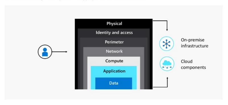
For instance, the cloud provider may ensure the physical security of the data centers, the integrity of the network, and the underlying infrastructure. On the other hand, the customer is often responsible for securing the data they store and process in the cloud, setting up secure access controls, and protecting their own networks and endpoints.
