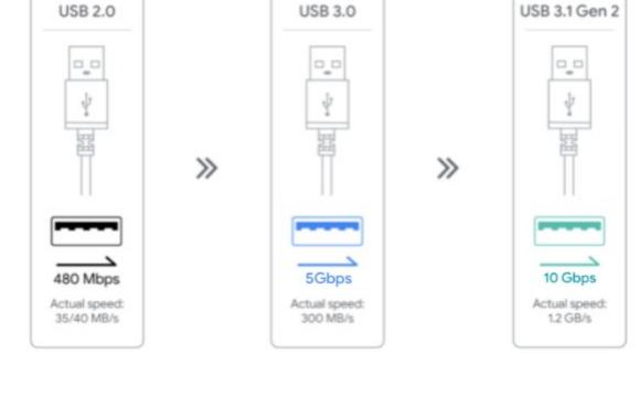
USB 2.0: Black port on the computer, 480 Mbps transfer speed USB 3.0: Blue port on computer, 5 Gbps transfer speed
